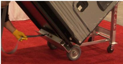
7. Slip the **Caster Plate** under the loose ratchet strap and hold it on the bottom of the load on the side directly opposite the Ultra Lift.
