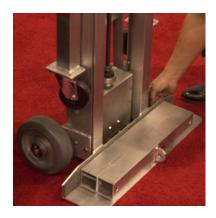
2. Tilt the load as you would with any hand truck and slide the Lift Plate/**Deck Plate** under the load.
