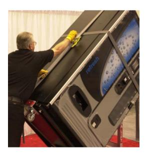
Note: An additional flap of strapping has been attached just behind the ratchet mechanism. Be certain that this strap is positioned between the ratchet mechanism and the load before tightening to prevent scratching the load.
