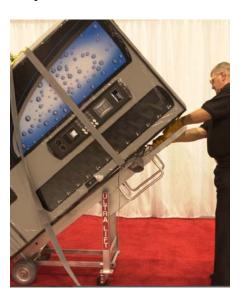
6. Pull the strap up and over the top of the load. Continue loosely strapping down the side of the load and around the bottom securing the second hook in the **Deck Plate** loop.
